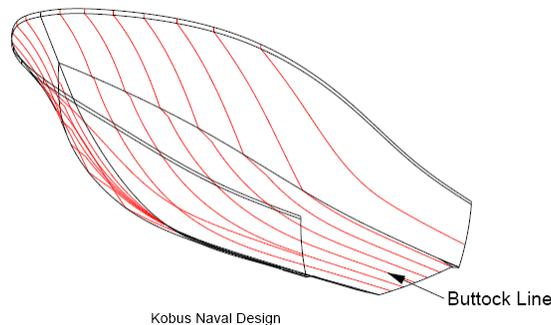
In the earlier years, many designers ran the spray rails along the buttock lines. (*Buttock Lines is a set of lines designers use to define the hull underbody. These lines are the curves that result from slicing the hull from top to bottom and front to back – like slicing your loaf of bread from end to end along the side. Experience designers can tell much about a boats potential performance from studying the buttock lines*).
